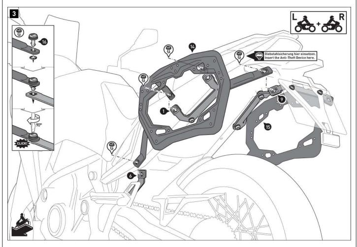
Connect the side carriers [14] and [15] to the quick-release fasteners and position [16] on mounting brackets [1], [2], [6] and [7] and the crossbar [9]. Secure the quick-release fasteners using the lock washers.
