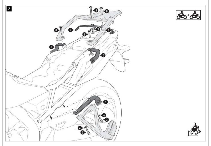
Screw the fastenings straps (1), (2), (5) and (6) as well as the crossbar (7) to both sides of the vehicle.
