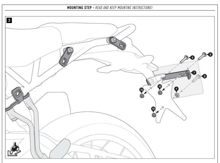
Screw the crossbar (7) to your license plate on the license plate holder. Do not tighten the screws yet.
