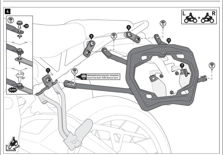
Using the quick-release fasteners, [13] connect the side carriers [11] and [12] to the mounting brackets [1] and [3] as well as to the crossbar [7]. Secure the quick-release fasteners using the lock washers.
