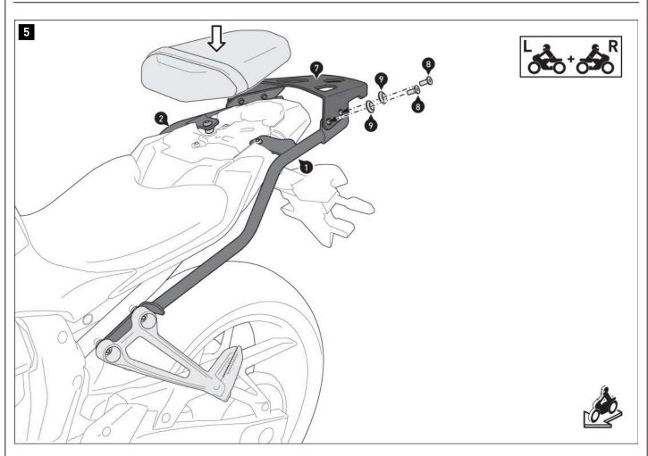
Screw the rack (7) onto mounting struts (1) and (2). **A WARNING: Use liquid threadlocker!** When all components have been loosely attached, tighten the screws (8) as specified in the mounting instructions. Tighten screws (4) and (6) according to the bike manufacturer's specifications.
