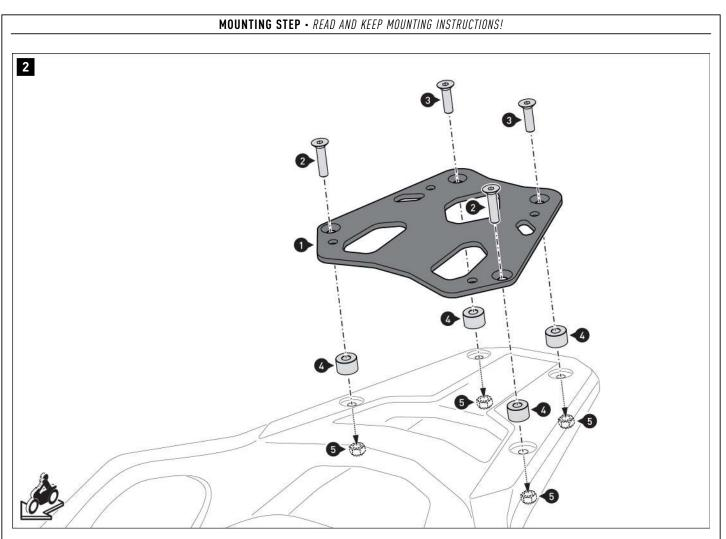
Mount the mounting bracket (1) on the rack. Tighten the screws as specified.
