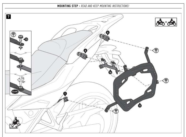
$\triangle$  **NOTE:** The SW-MOTECH anti-theft protection devices are available separately; mount the anti-theft protection devices on both sides at the indicated position. a
