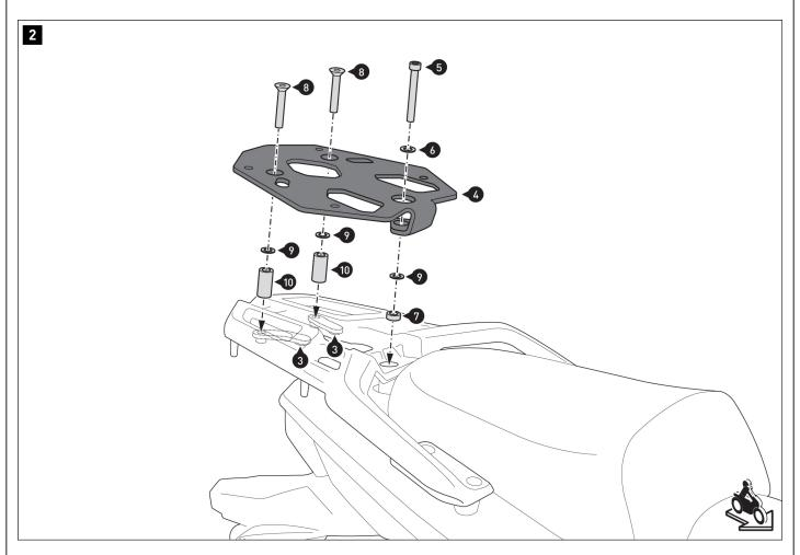
Mount the mounting bracket (4) on the rack.
