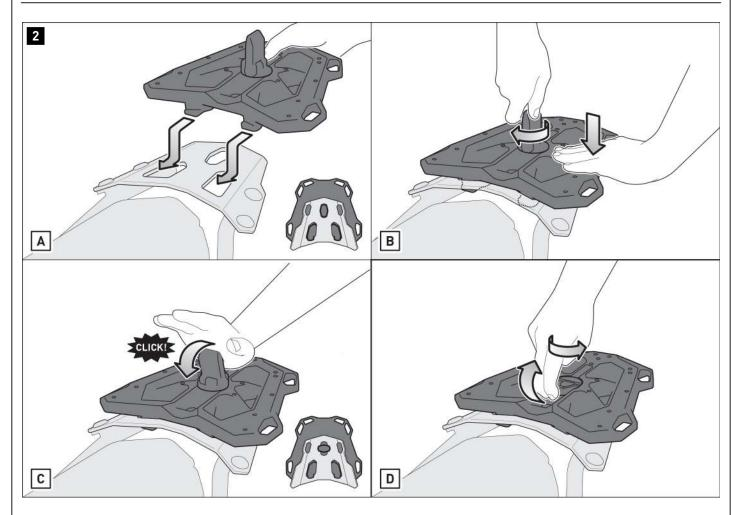
**Figure [A]:** Slide the adapter plate (1) with the two hooks into the openings of your STREET-RACK (sold separately).
