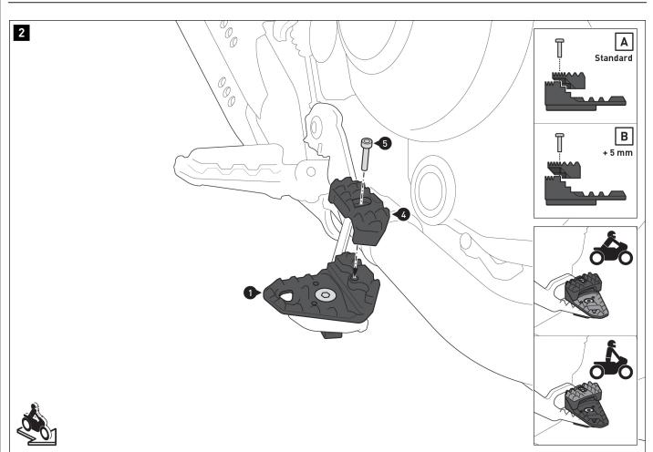
Screw the riser (4) onto the extension (1) in position [A] (standard) or [B] (+ 5  $\,$ mm). **A WARNING: Use a liquid threadlocker!** Tighten the screw as specified in the mounting instructions.
