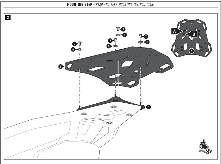
$\triangle$  **NOTE:** Depending on the space available, screw the rack (6) to the marked mounting position (A) or(B) as shown in the detailed drawing.
