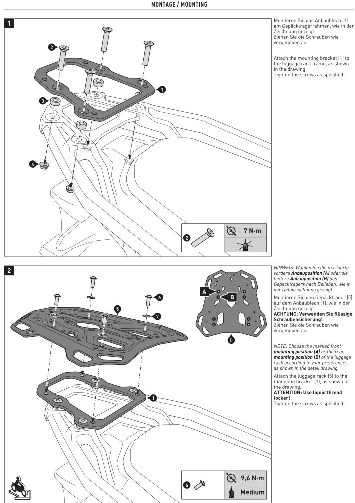
Attach the mounting bracket (1) to the luggage rack frame, as shown
