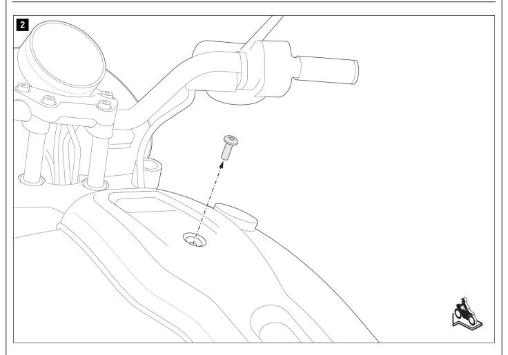
Remove the original screw from the vehicle.
