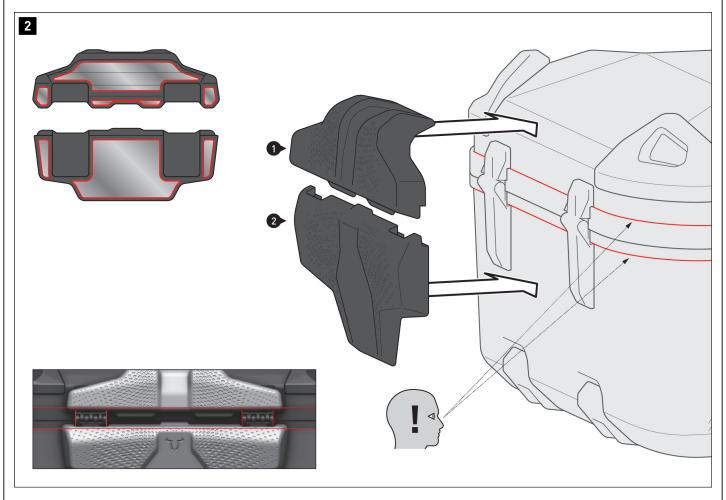
$\triangle$  **NOTE:** Before gluing, determine the exact position of the passenger backrests (1/2) on the lid and body of your DUSC. Ensure they rest securely on the frame profiles (marked in red; see lower left and right illustrations).
