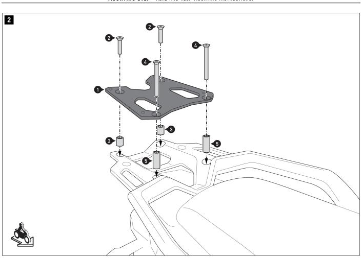
Mount the mounting bracket (1) on the rack. **A WARNING: Use a liquid threadlocker!** Tighten the screws according to the manufacturer's instructions.
