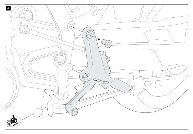
Loosen the screws shown, and remove the left footrest system from the bike.
