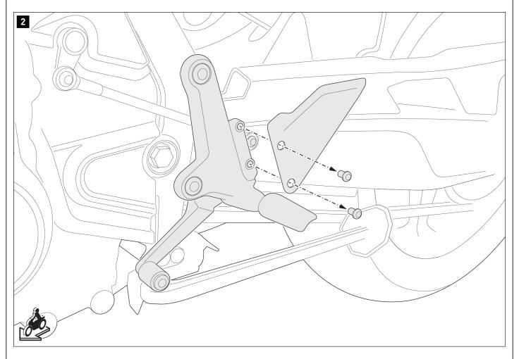
Loosen the screws shown and remove the heel guard from the left footrest.
