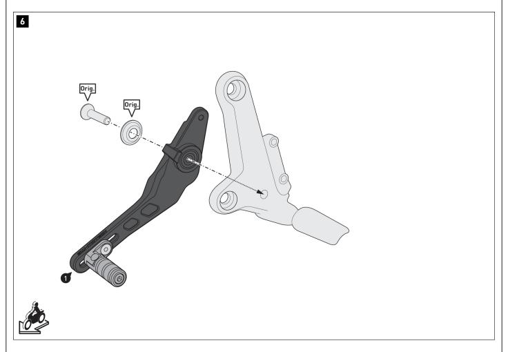
Screw the gear lever (1) onto the footrest system.
