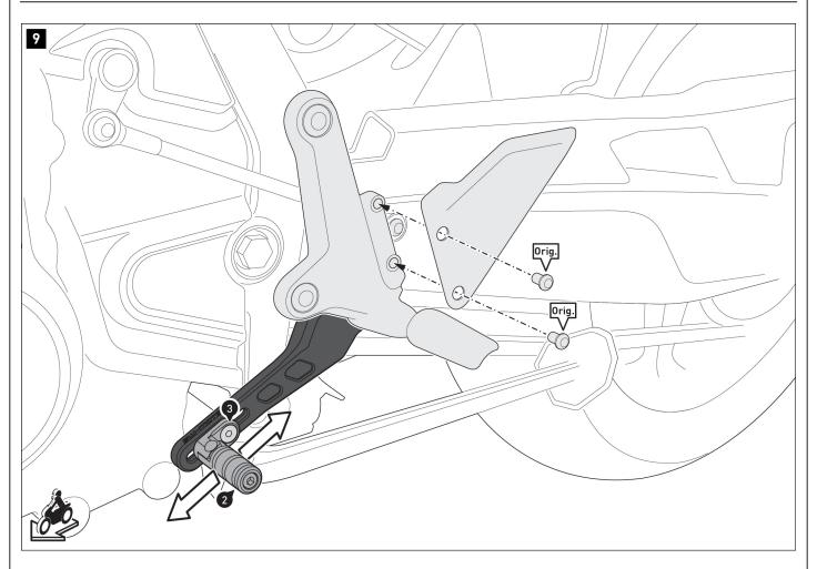
Screw the heel guard back onto the left footrest.
