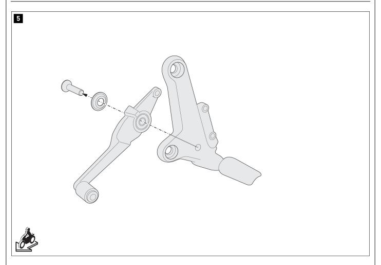
Remove the original gear lever from the footrest system.
