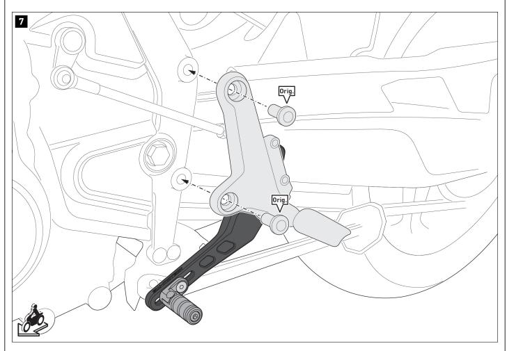
Reinstall the footrest system on the bike.
