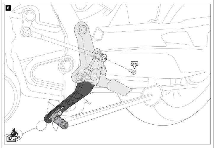
Screw the gear shift linkage to the brake pedal.
