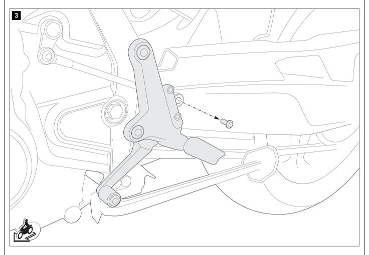
Remove the screw shown from the gear shift linkage.
