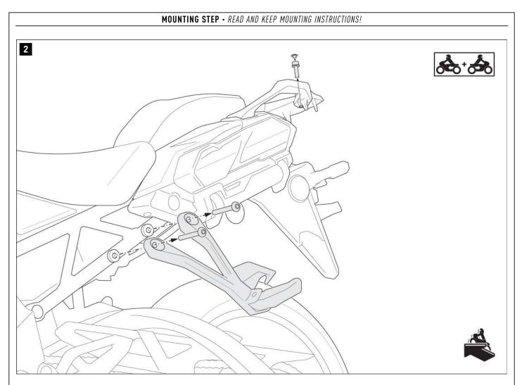
Remove the screws shown **on both sides** and the passenger footrest holders from the vehicle.
