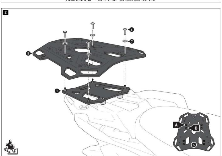
▲ **NOTE:** Depending on the space available, screw the rack to **mounting position** (A) or (B), as indicated in the detailed drawing.
