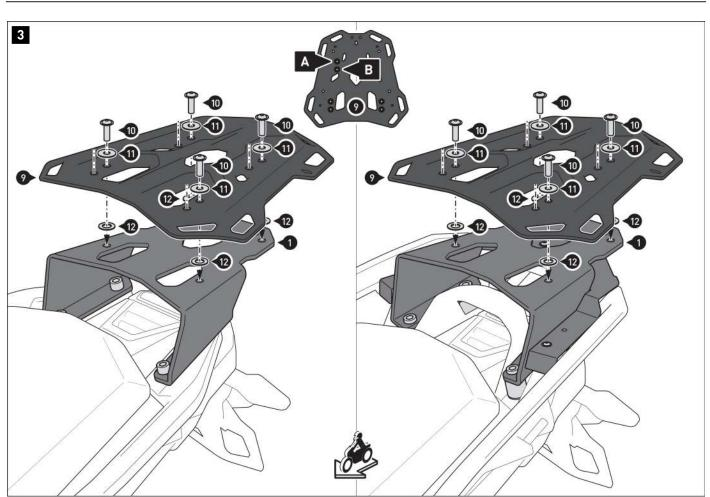
▲ **NOTE:** Depending on the space available, screw the rack to the marked**mounting position (A)** or **(B)** , as shown in the detailed drawing .
