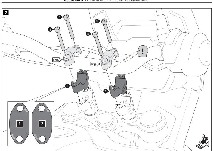
To align the handlebars, use the cross on the handlebars as a guide, if available.
