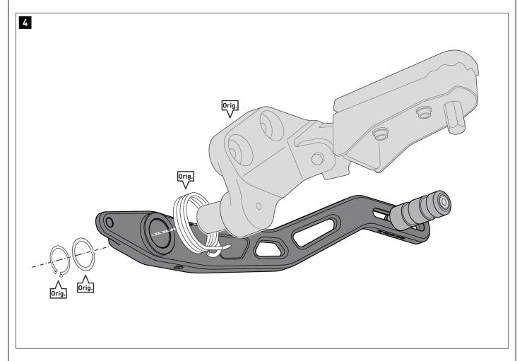
Mount the brake pedal onto the footrest system using the original parts (Orig.).  $\label{eq:control} % \begin{subarray}{ll} \end{subarray} % \be$
