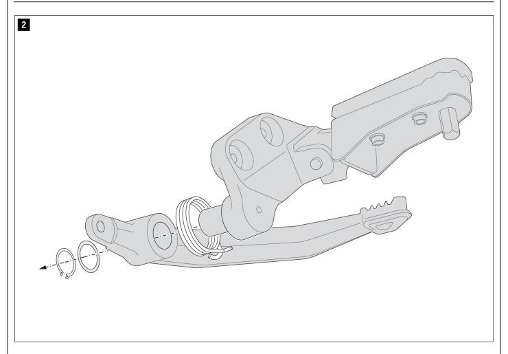
Loosen the circlip from the footpeg system mount. Then remove the original brake pedal.
