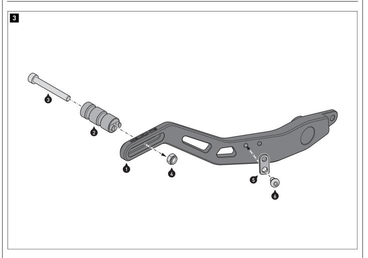
Screw the parts shown together. **A** WARNING: Use liquid thread locker for screw (6)!
