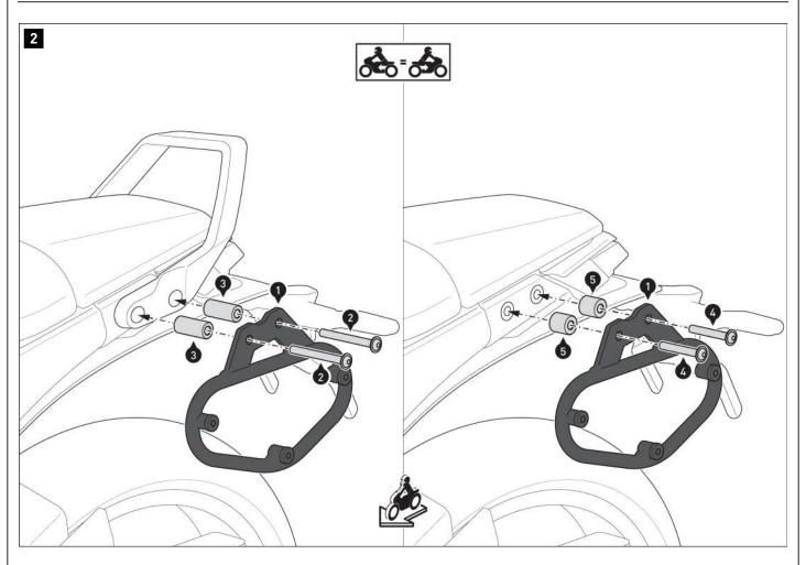
Screw the side carrier [1] to the vehicle using the parts indicated. **A** WARNING: Use a liquid threadlocker!
