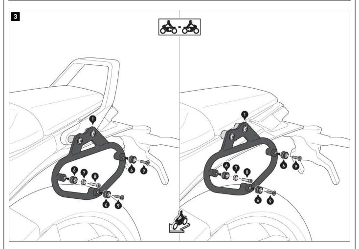
Screw parts [6] to [9] to the side carrier [1].
