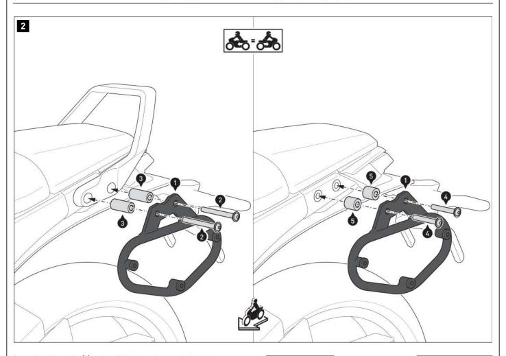
Screw the side carrier [1] to the vehicle using the parts indicated.
