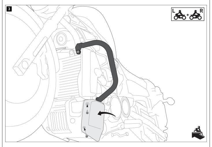
Install the original covers (Orig.) on the vehicle using the original screws (Orig.).
