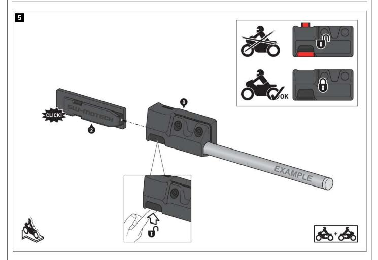
Slide the connectors (8/9) onto the connector rails (2/3) on both sides.
