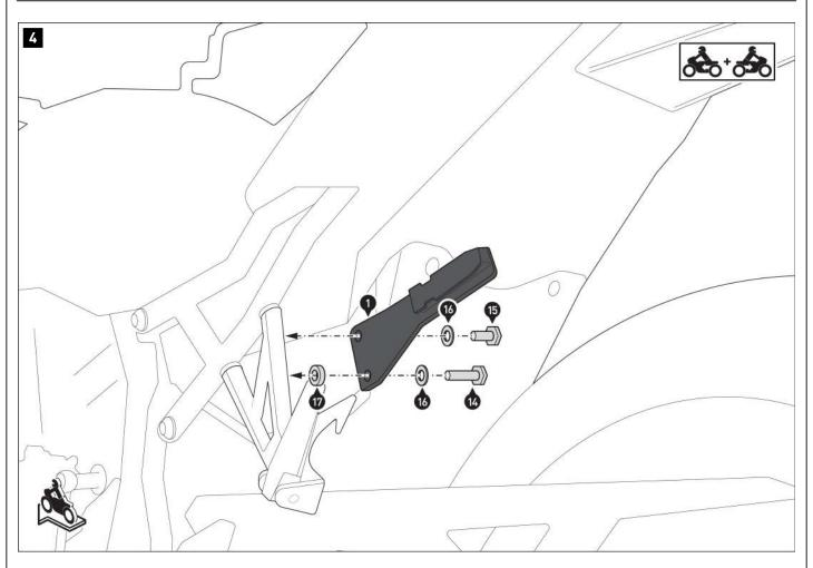
Screw the mounting brackets (1) to the passenger footrest mounts. **A** WARNING: Use a liquid threadlocker!
