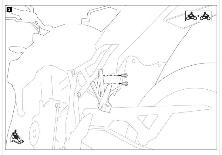
Remove the original screws shown from the vehicle.
