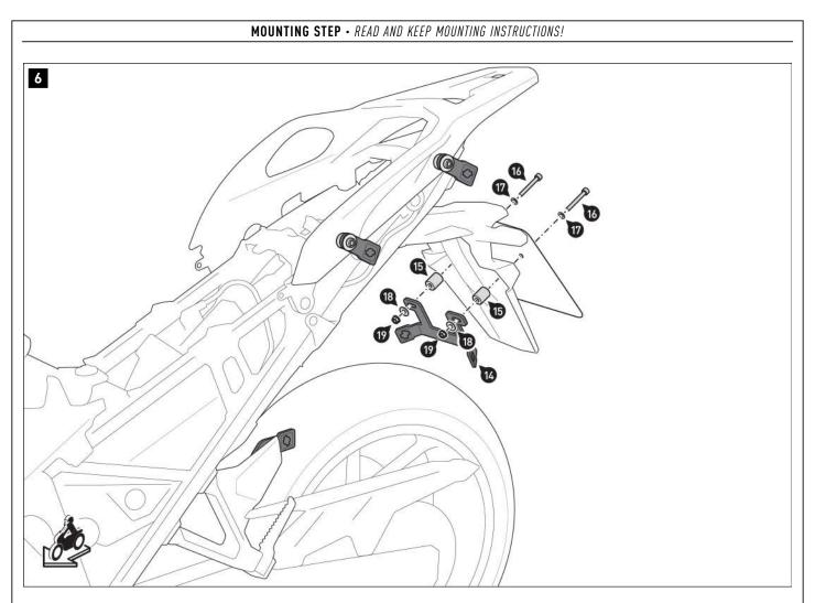
Screw the crossbar (14) to the license plate on the license plate holder. Do not tighten the screws (16) yet.
