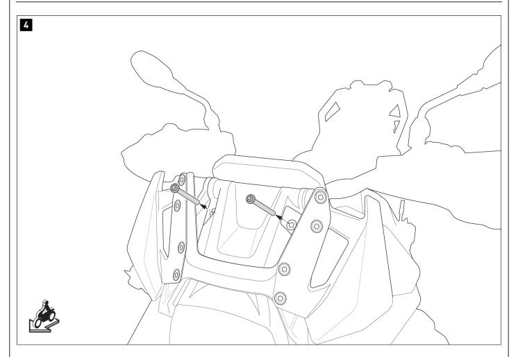
Loosen the two screws shown.
