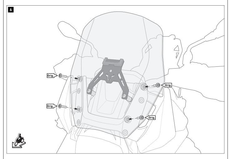
Screw the windscreen onto the vehicle using the original screws (Orig.). Tighten the original (Orig.) screws according to the manufacturer's instructions.
