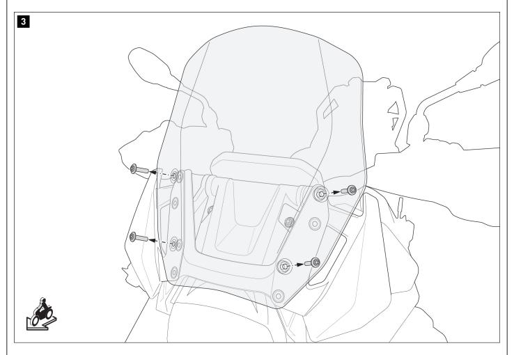
$\triangle$  **NOTE:** The windscreen holders are only plugged in and can fall down after dismantling the windscreen.
