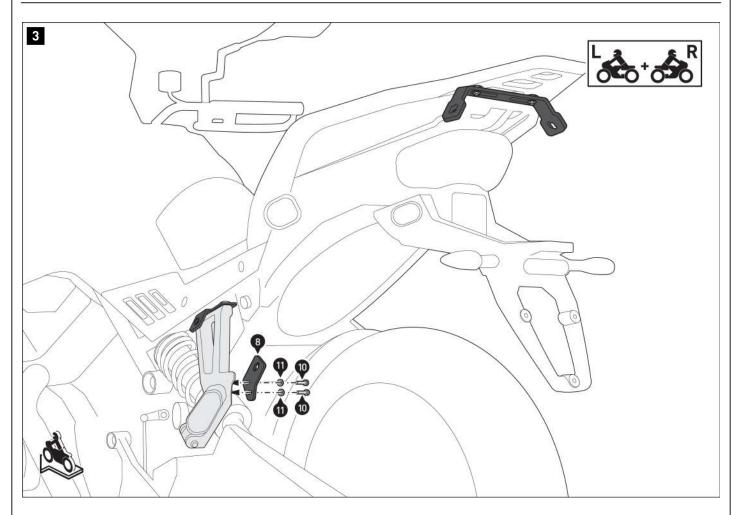
Screw the fastening tabs (8/9) **onto both sides** of the pillion footrest holders. **A WARNING:** Use a liquid threadlocker!
