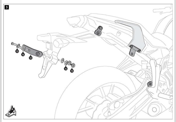
Screw the crossbar (12) to the license plate holder. Do not tighten the screws yet.
