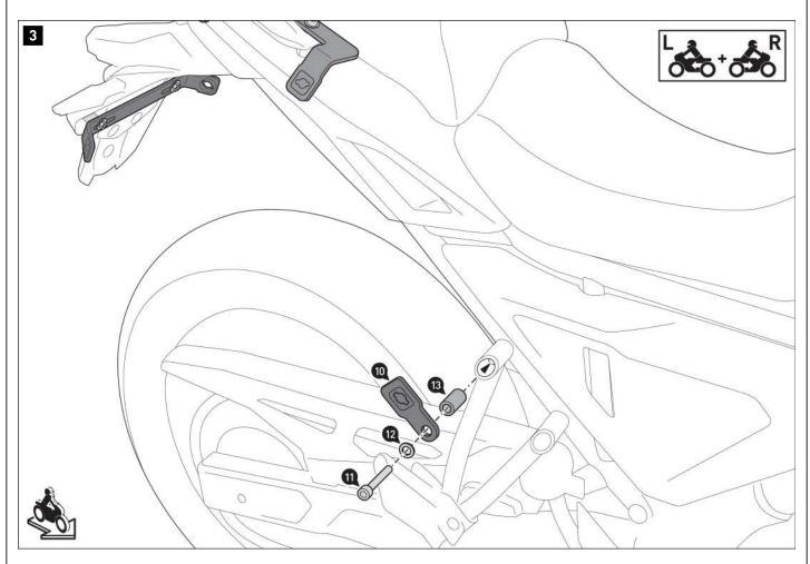
Screw the mounting brackets [10] onto each of the passenger footrest  $% \left( 10\right) =100$
