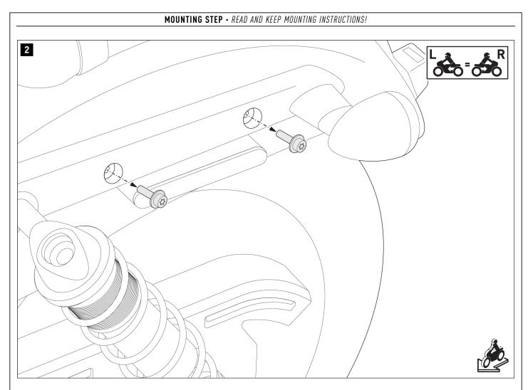
Remove the screws indicated from the vehicle.
