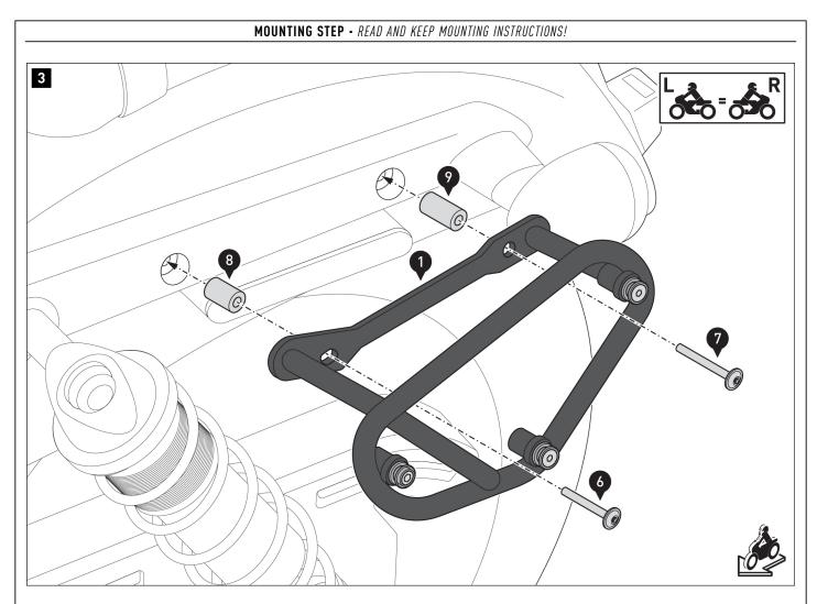
Screw the side carrier (1) to the vehicle. **A WARNING: Use a liquid threadlocker!** Tighten the screws according to the manufacturer's instructions.
