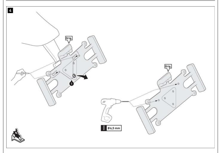
Use a suitable tool to mark the two drilling points on the back of the license plate holder (Orig.).
