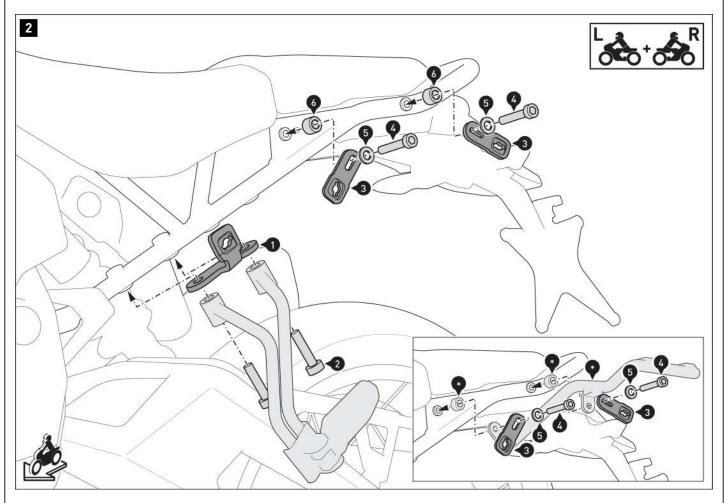
Screw the mounting brackets [1] to the passenger footrests on both sides of the vehicle. **AWARNING:** Use a liquid threadlocker!
