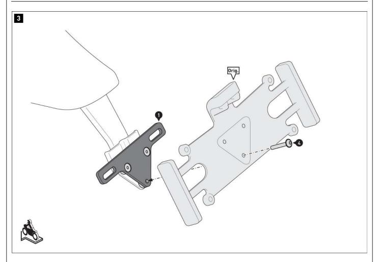
Screw the original license plate holder (Orig.) loosely onto the vehicle with the screw (4). Do not tighten the screw (4) yet.
