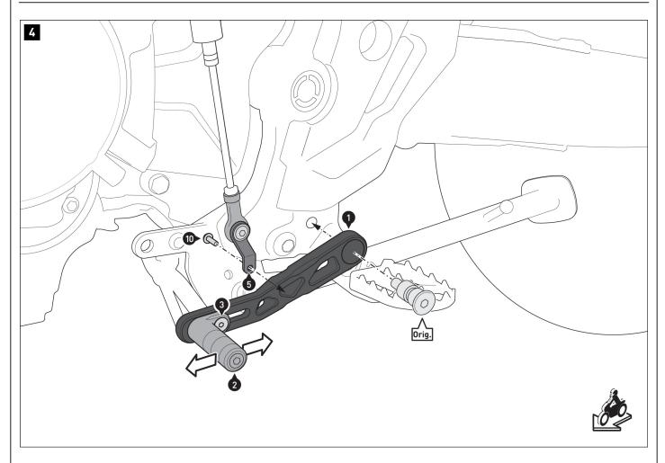
Screw the gear shift rod plate (5) to the gear lever (1). **A** WARNING: Use a liquid threadlocker!
