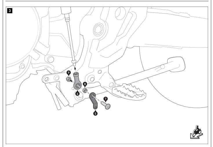
Screw the parts shown together. Then tighten the screw (7) as specified in the mounting instructions.
