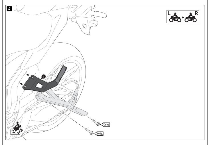
Screw the mounting bracket (1/2) to the vehicle.
