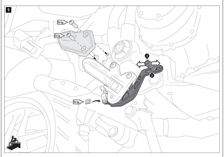
Screw the footrest system back onto the vehicle.
