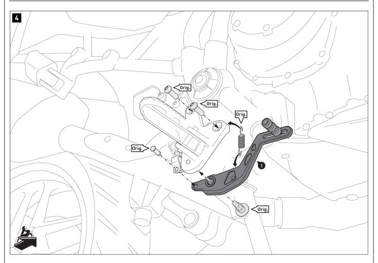
Hang the spring as well as the cradle suspension (5) on the vehicle and screw the brake pedal (1) to the footrest system using the original parts (Orig.).
