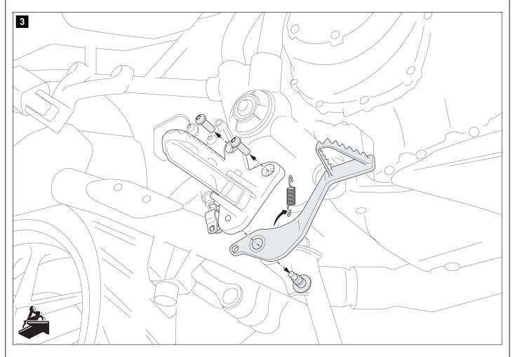
Loosen the indicated screws and unhook the spring.
