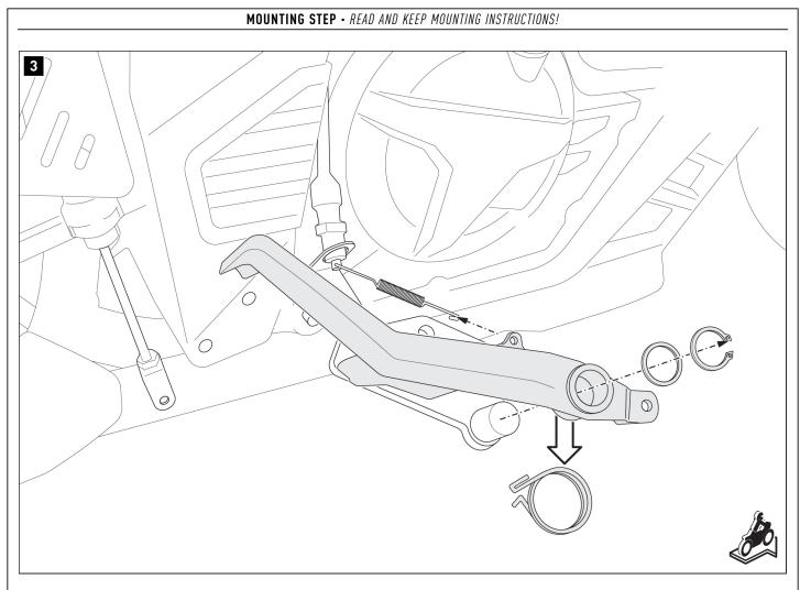
Loosen the locking ring and remove the original brake pedal.
