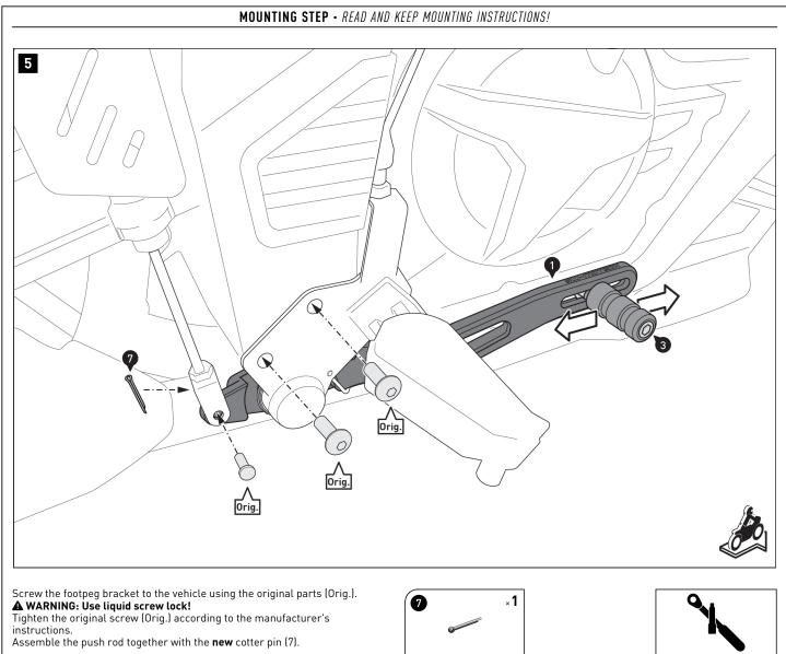
Adjust the pedal according to your driving habits. Then tighten the screw (3) as specified in the instructions.
