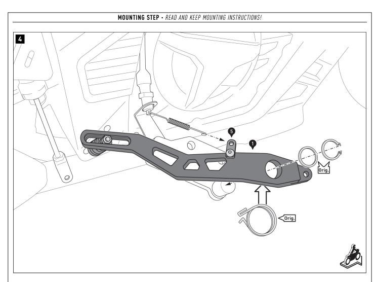
Assemble the brake pedal (1) together with the original parts (Orig.) on the footpeg bracket. Position the original spring (Orig.) as it was mounted on the original gear lever.
