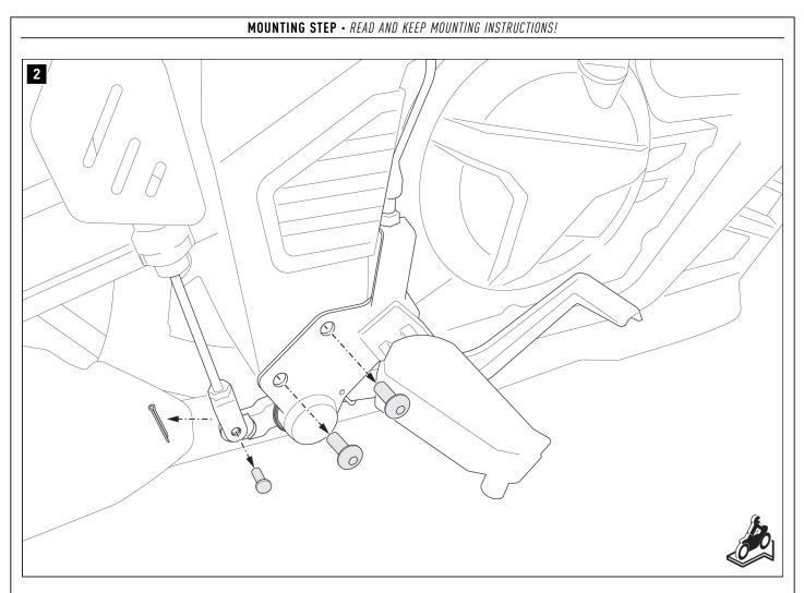
Remove the cotter pin and screws from the footpeg bracket.
