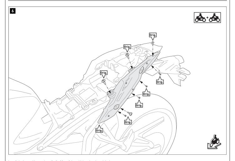
Install the inner side panels on **both sides** of the vehicle using the original screws/plastic dowels.
