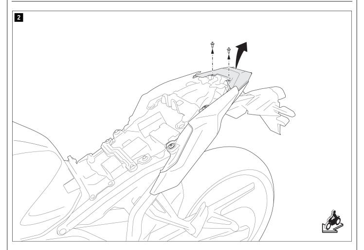
Loosen the two plastic dowels, and remove the rear panel from the vehicle.
