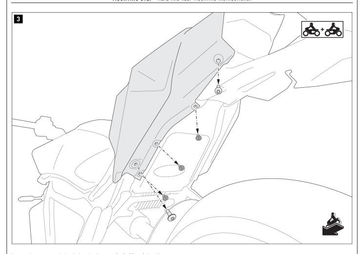
Loosen the screws and plastic dowels shown on  ${\bf both\ sides}$  of the side panelling.
