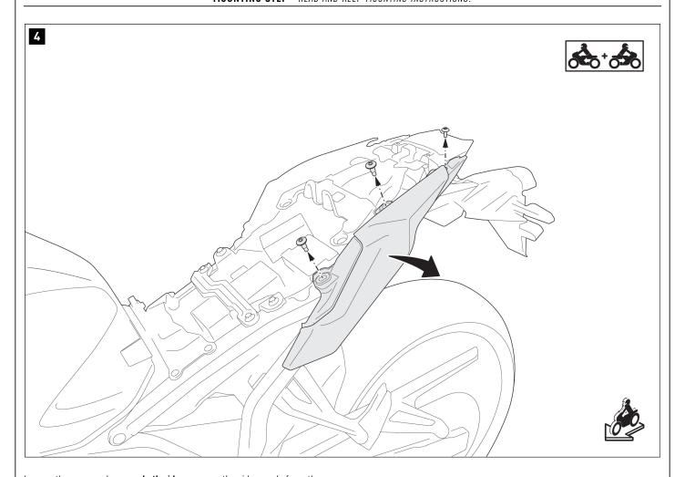
Loosen the screws shown on  ${\bf both\ sides};$  remove the side panels from the vehicle.
