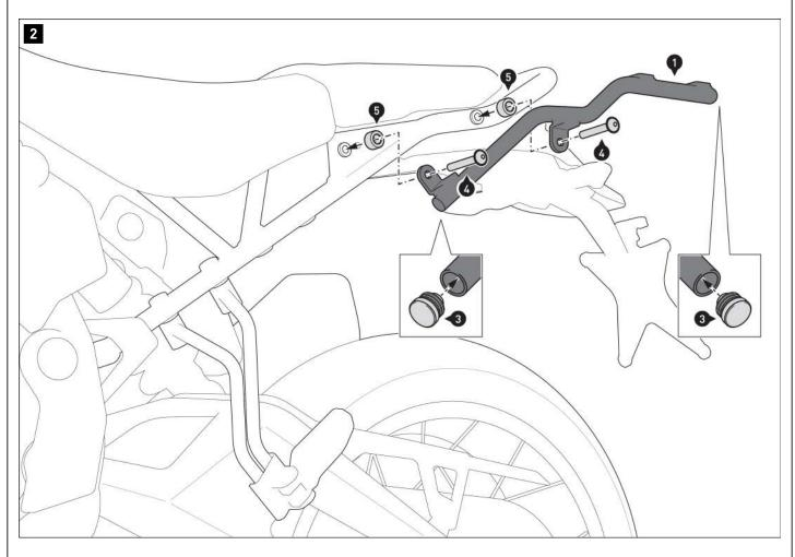
Insert the plastic plugs (3) into the ends of mounting struts (1) and (2).
