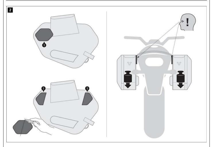
Check the correct positioning of the abrasion/edge protectors (1) again once the BLAZE saddlebags have been loaded.
