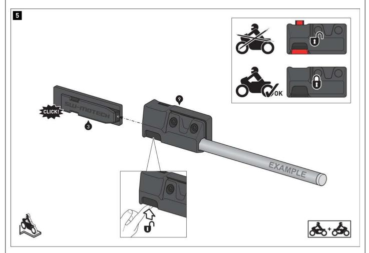
Slide the plug connectors (9/10) onto the connector mounting rails (3/4) on
