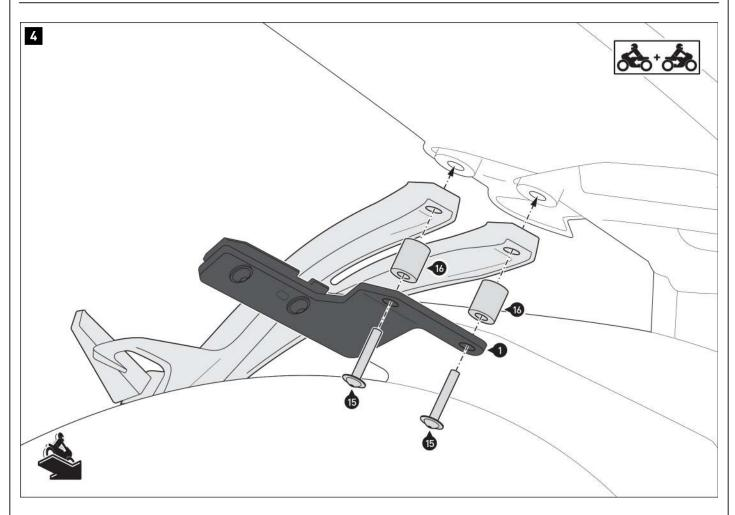
Screw the mounting brackets (1/2) to the passenger footrest holders on the vehicle.
