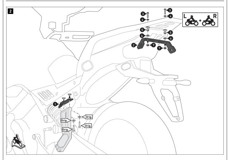
Screw the fastening tabs (1)  ${f onto}$   ${f both}$   ${f sides}$  to the pillion footrest holders on the vehicle.
