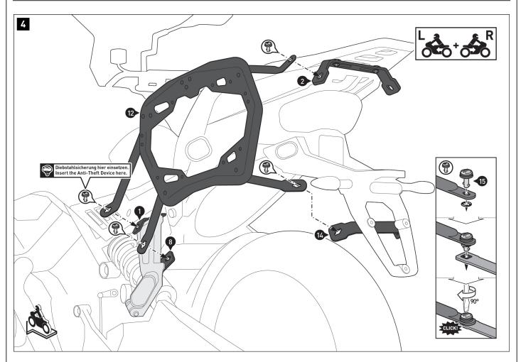
$\triangle$  **NOTE:** SW-MOTECH anti-theft protection is sold separately; mount the anti-theft protection devices on both sides at the marked position.
