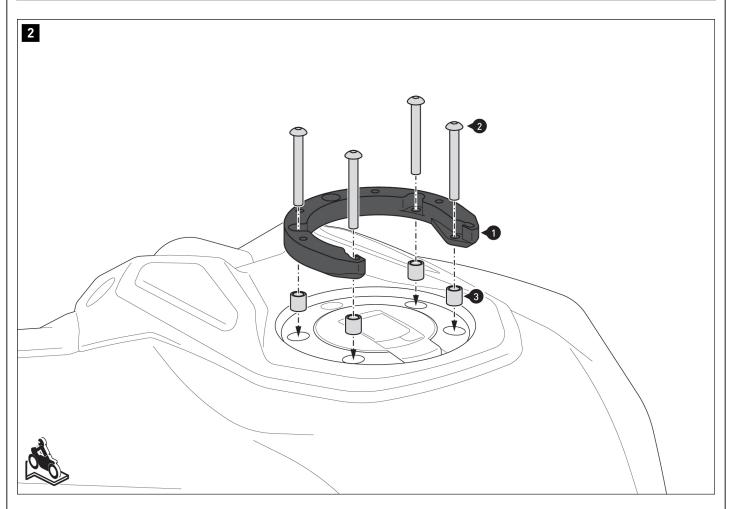
Screw the mounting ring (1) onto the tank cap ring. **A** WARNING: Use a liquid threadlocker!
