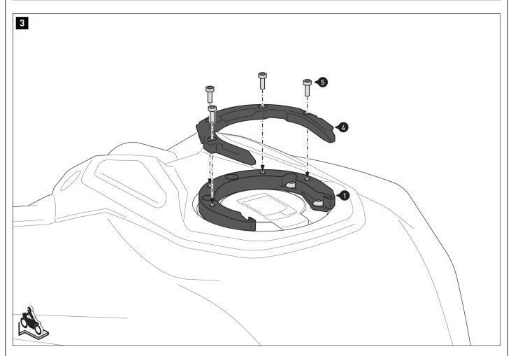
Carefully screw the tank ring (4) to the mounting ring (1).
