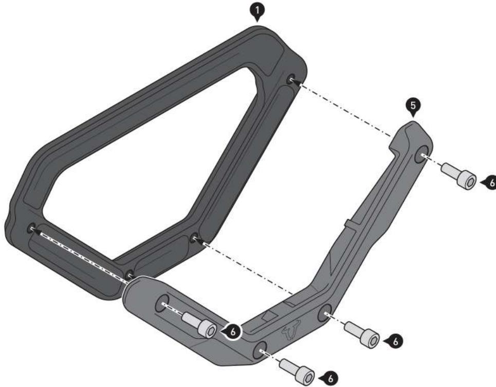
Screw the base (5) to the side carrier (1).
