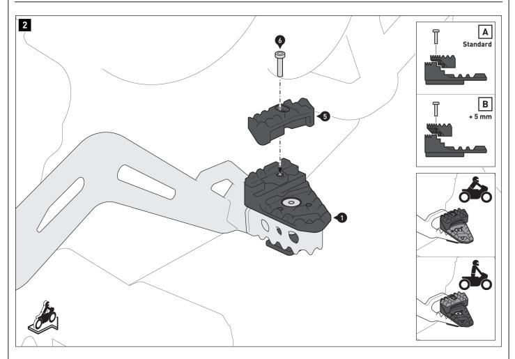
Screw the riser (5) onto the extension (1) in position [A] (standard) or [B] (+ 5  $\,$ mml.
