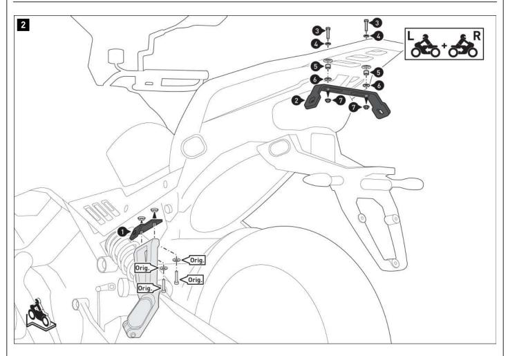
Screw the fastening tabs (1)  ${f onto}$   ${f both}$   ${f sides}$  to the pillion footrest holders on
