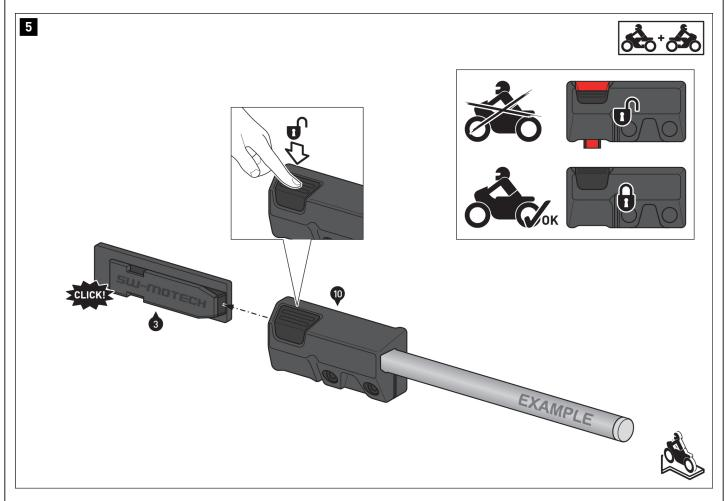
Slide the connectors (10/11) onto both sides of the connector mounting rails (3/4).
