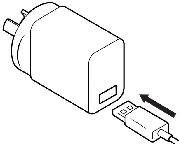
Plug USB cable into an 10W or higher power supply.
