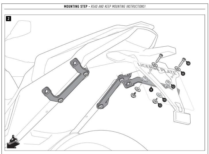
Screw the crossbar (9) to your number plate on the license plate holder. Do not tighten the screws yet.
