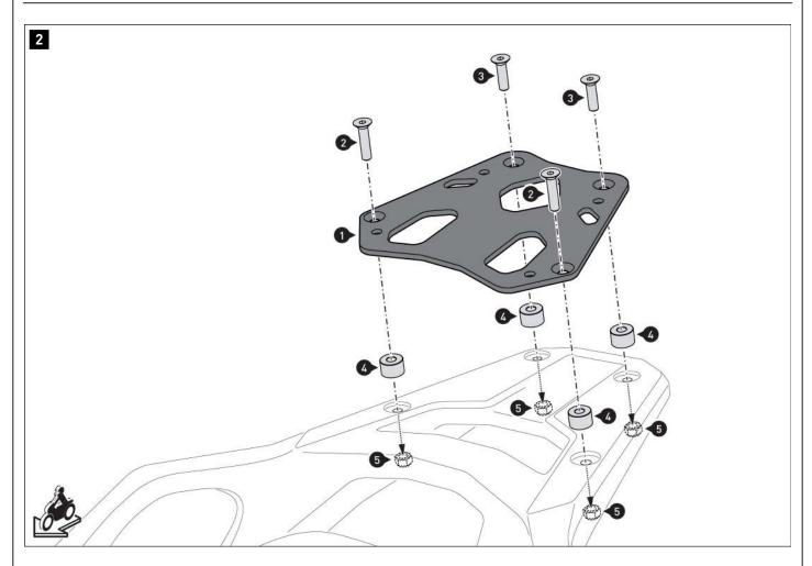
Mount the mounting bracket (1) on the rack. Tighten the screws as specified.
