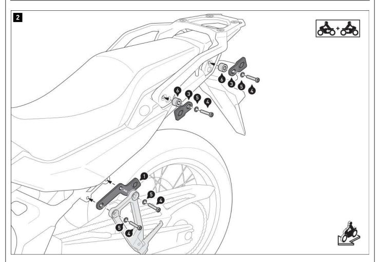
Screw the fastening straps (1), (2) and (3) to both sides of the vehicle.
