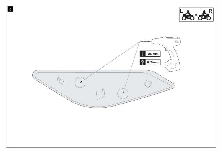
First, use a 6 mm drill bit to drill a pilot hole in the center of each of the circular markings on the fairing.
