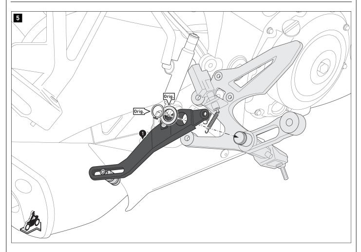
Install the foot brake lever (1) on the footrest bracket using the original parts (Orig.).
