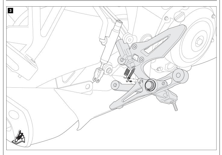
$\triangle$  **NOTE:** Before removing the original brake pedal, make a note of the position of the original springs.
