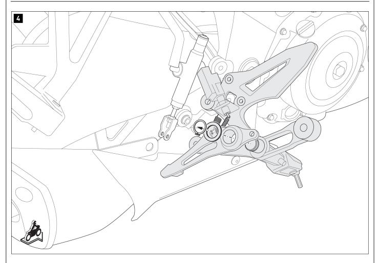
Remove the original brake pedal from the footrest mount.
