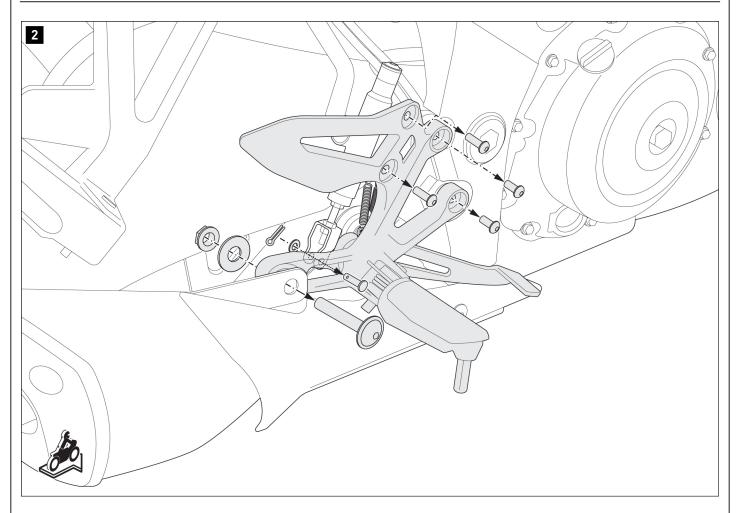
Loosen the cotter pin from the master cylinder push rod. Remove the parts shown from the right footrest mount.
