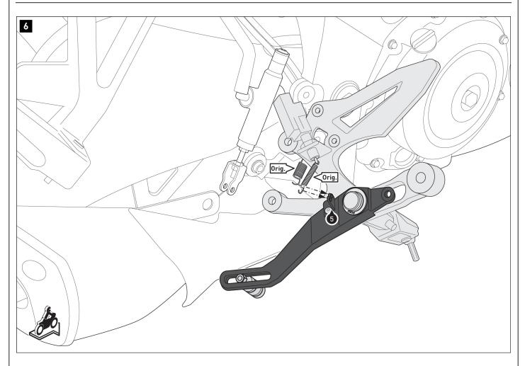
Hang the original springs (Orig.) into the spring plate (5) as they were attached to the original brake pedal.  $\label{eq:continuous}$
