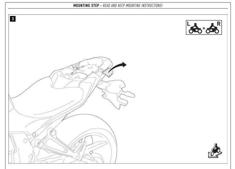
Remove the fairing from the  ${\bm left}$  side of the vehicle.
