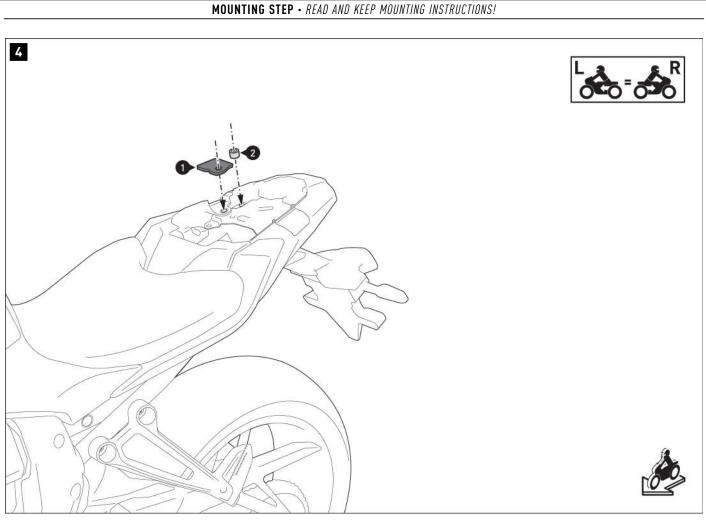
Place the mounting bracket (1) on the middle mounting point and the spacer (2) on the rear mounting point of the vehicle frame.
