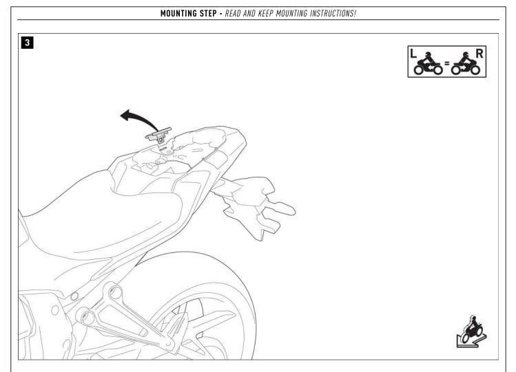
Remove the fairing from the  ${\bf right}$  side of the vehicle.
