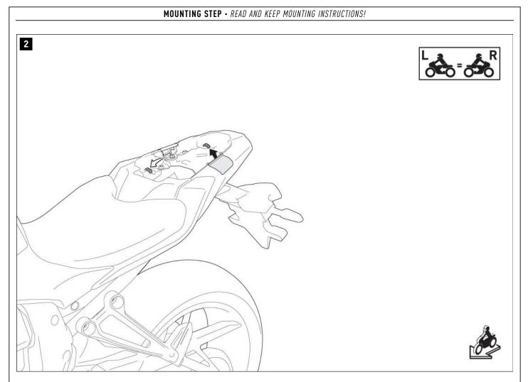
$\triangle$  NOTE: Disassembly of the right plastic clip is not necessary and is shown only for better understanding.
