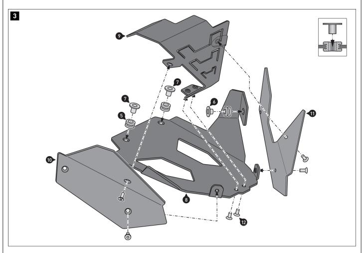
Insert the rubber grommets (5) into the holes in the bottom of the engine guard (8).
