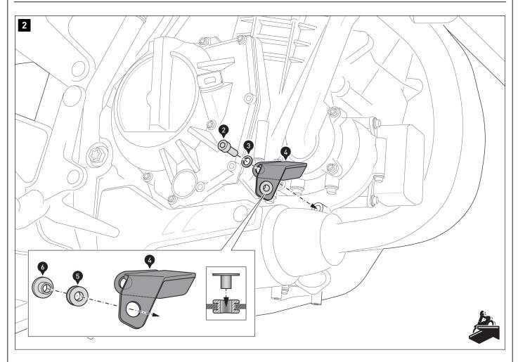
Insert the rubber grommet (5) into the hole shown in the mounting bracket (4).
