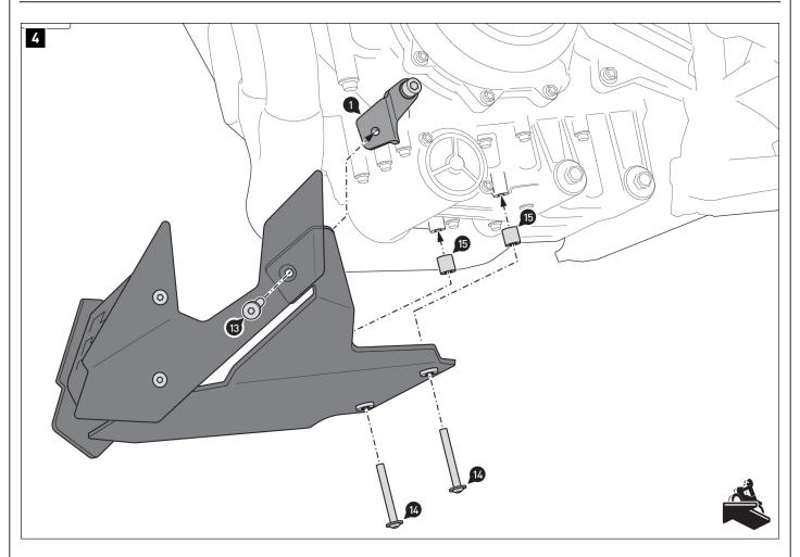
Screw the engine guard to the mounting bracket (1) and to the vehicle. **A WARNING:** Use a liquid threadlocker!
