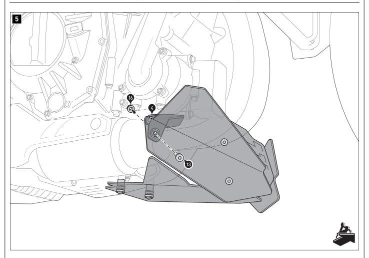
Screw the engine guard to the mounting bracket (4). **A WARNING: Use a liquid threadlocker!**When all components are seated without tension, tighten the screws (2, 13, and 14) as specified in the mounting instructions.
