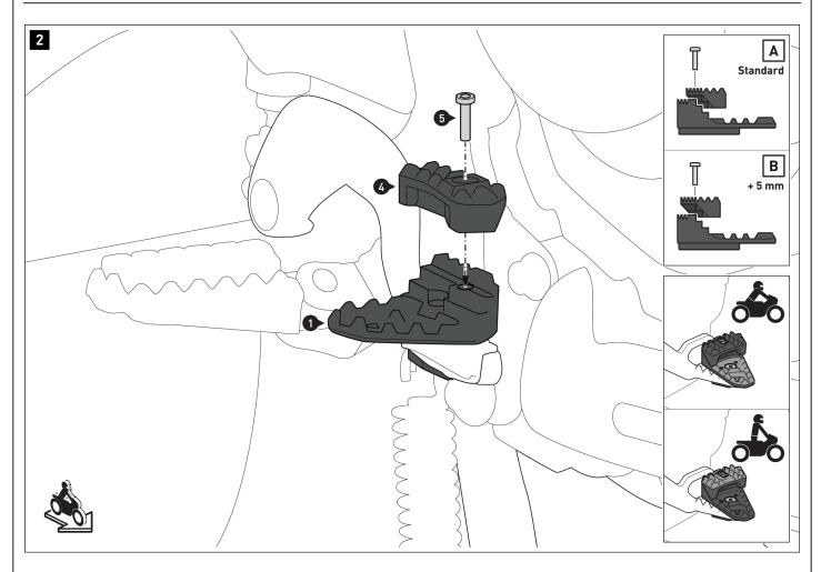
Screw the riser (4) onto the extension (1) in position [A] (standard) or [B] (+ 5mml.
